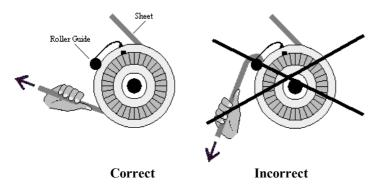
When **pulling-in sheets**, the gear ring must be set to the "black" position. In this mode the Setamar winch behaves like a conventional two-speed self-tailing winch, i.e. when the handle is turned in the normal direction the gear ratio is 1:1 and when the handle is turned in the reverse direction the sheet will be hauled in at a lower gear.
